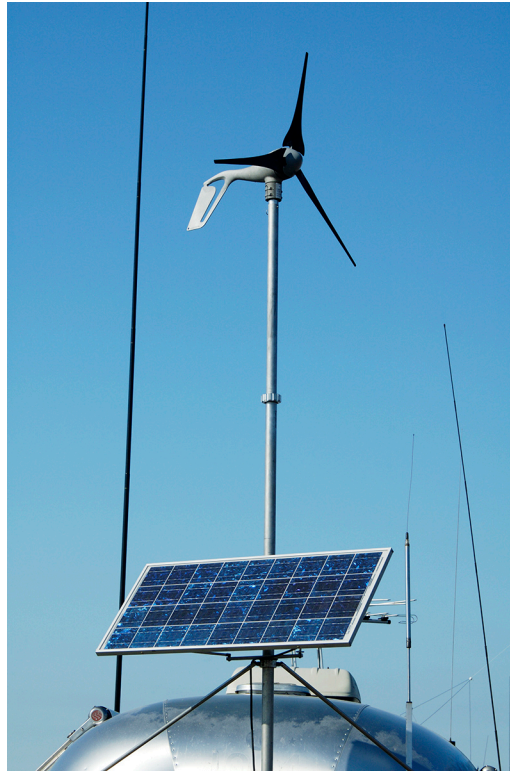
Figure 19. In recreational vehicles, a wind turbine can be used to supply electricity to dc powered devices and keep the battery charged. The recreational vehicle pictured above also uses a solar panel to produce electricity.
