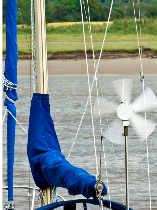
Figure 18. Sailboat equipped with a stand-alone wind power system.
